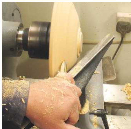
▲ Pic.8 If you look at the profile of the bowl you can see the ogee shape that Les is after. If you take lighter pull cuts a better surface finish will be achieved
